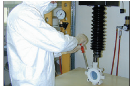
Valve assembly in clean room
